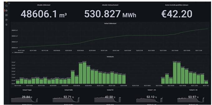
Abb. 1: Software die den Verbrauch der Heizungsanlage darstellt. Fig. 1: Software that displays how much energy the heating system is using.
